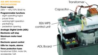
230V~ +6%/-10% 50-60 Hz single phase, bi-directional. 400W 2A 500N (Z20) 1400 rpm 135°C
