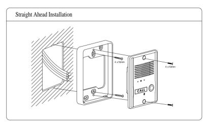
After attach the body supporter with 2 screws, put the Door Camera into the grooves of body supporter, and then fix it with 2 screws and stick the finishing materials.
