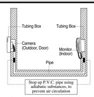
X Stopping up pipe as above minimizes temperature difference between indoors and outdoors, and also eliminates moisture and condensation on door camera window.
