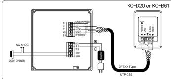
In case of UPT cable wiring, please refer to the wiring and this wiring is recommended. please avoid wiring R(audio)and W(video) in a twisted cable.
